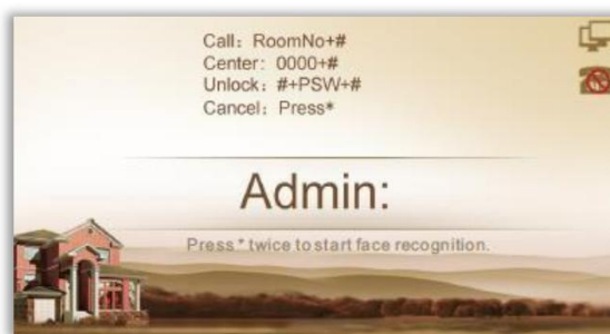
Figure 11: LCD interface section of the Outdoor Panel
