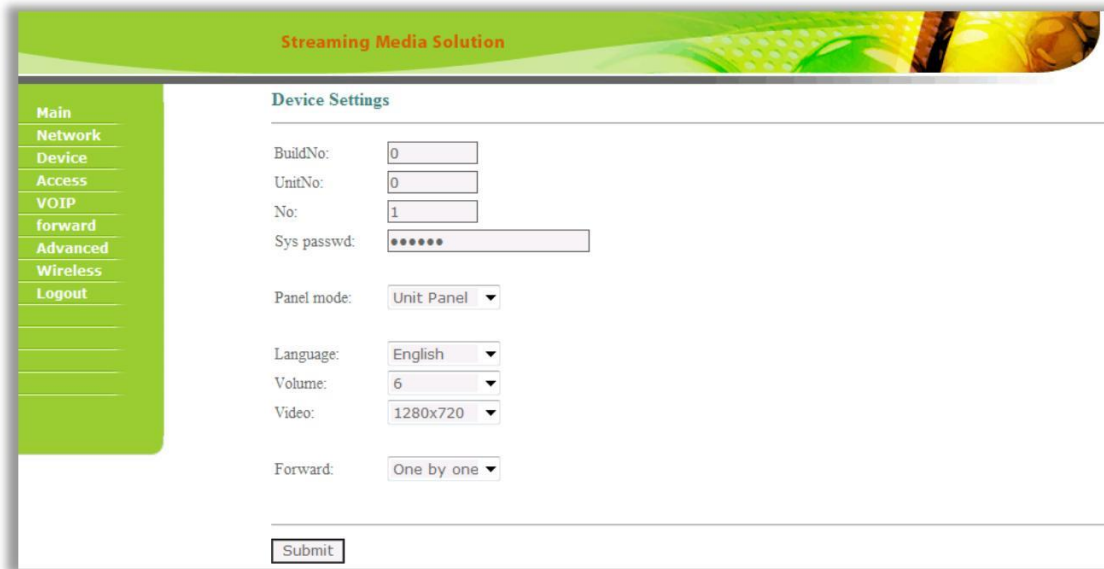
Figure 25: Device Settings Interface of the Outdoor Intercom
