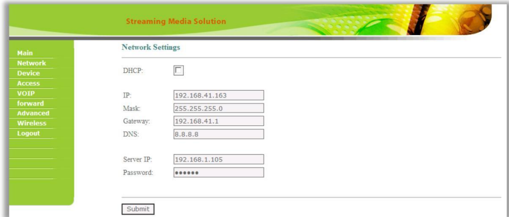
Figure 24: Web Settings network interface of the Indoor Panel
