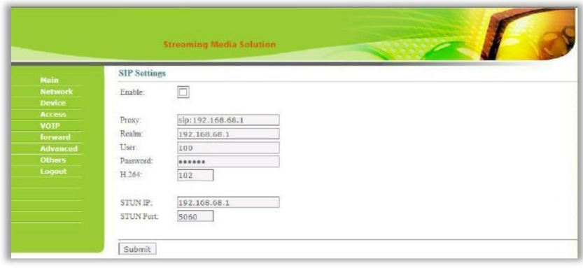
Figure 27: SIP Settings interface of the outdoor intercom
