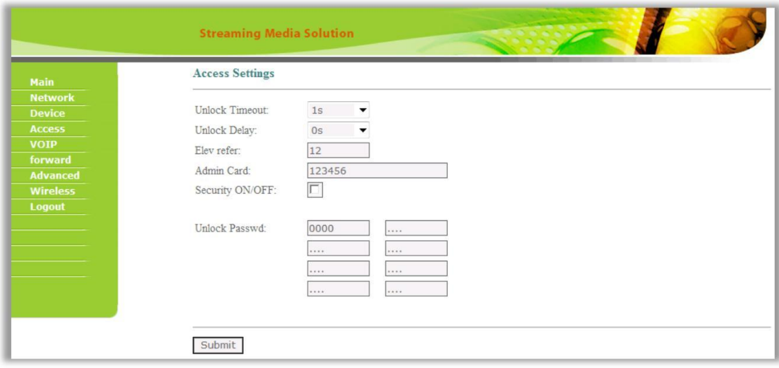
Figure 26: Web Access Settings interface
